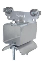
**Product Code** Wheel Steel roller VS1032P5-105/6 | Material Carrier body steel Support saddle steel Hardware galvanized Temperature resistance -30°C to +70°C Max. Cable Load 16 kg per carrier
