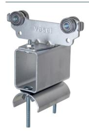
**Product Code** Wheel Steel roller VS1032P5-105/4 Material Carrier body steel Support saddle steel Hardware galvanized Temperature resistance -30°C to +70°C Max. Cable Load 16 kg per carrier
